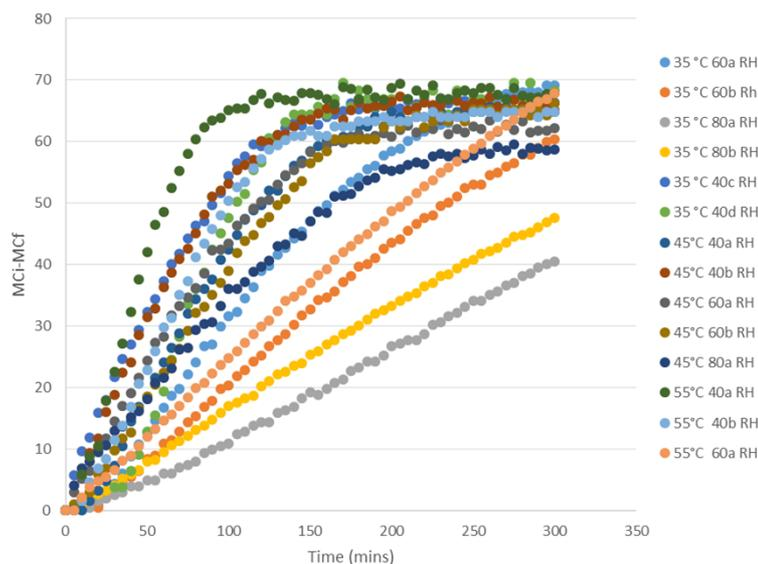
Figure 1: Graphical representation of all three temperatures (35, 45, 55°C) at varying humidity.
