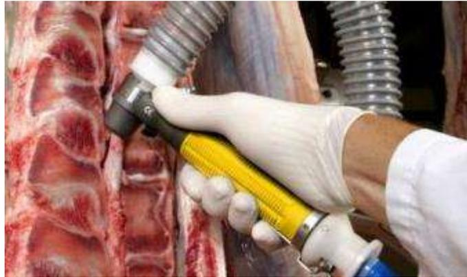
**Fig. 2** The image shows one of the tools that is currently used manually to remove the spinal cord from beef sides. It consists of a circular rotating cutting blade that gets in behind the spinal cord and cuts the Dorsal Root Ganglia before vacuuming away the removed material.
