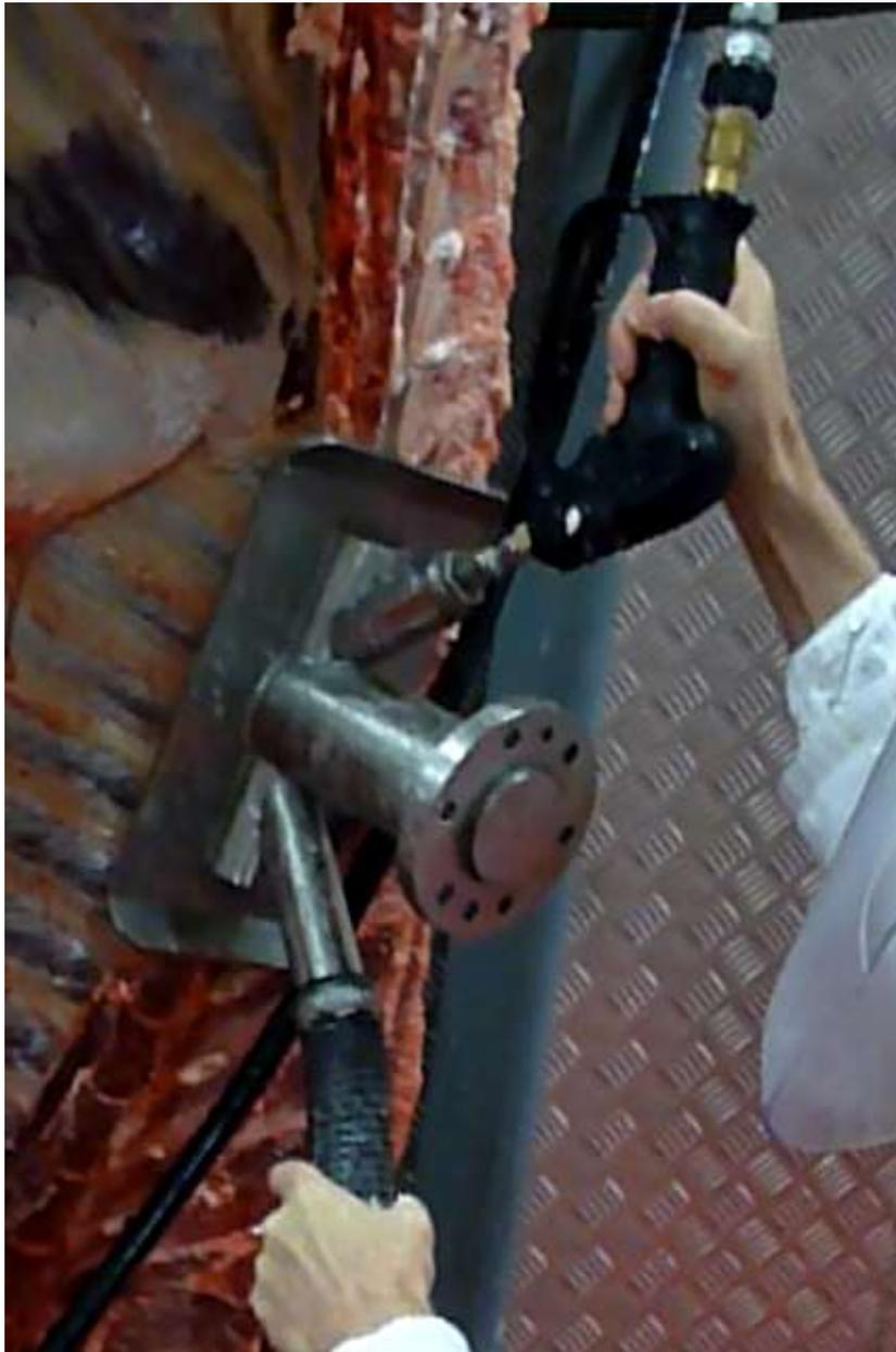
**Fig.4** This image shows the Robotic spinal cord removal tool developed during past trials. The high pressure water enters from the top and the spinal cord and water are removed by vacuum at the bottom of the tool.
