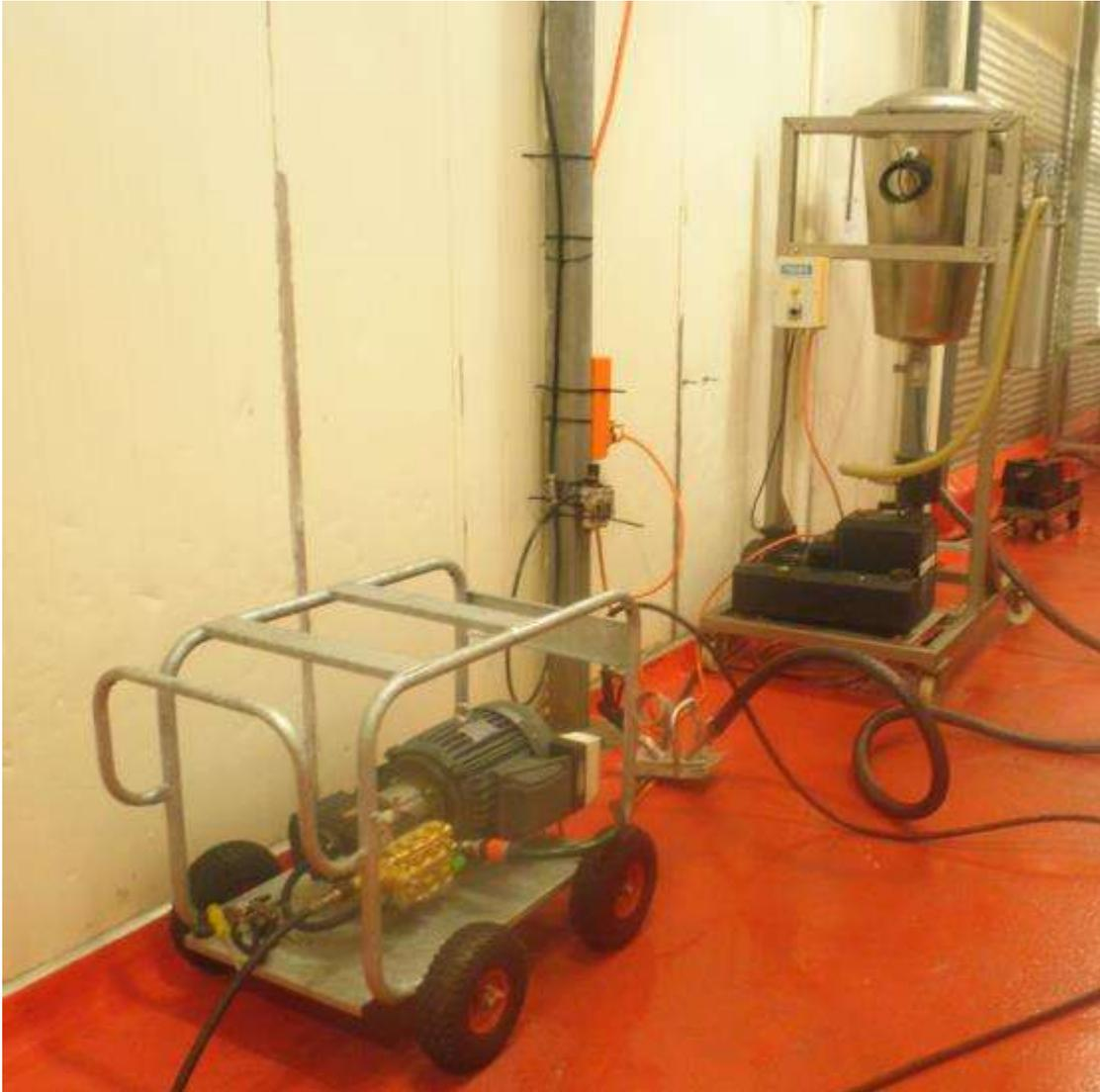
**Fig. 3 High pressure water unit and vacuum unit ready to conduct trials and testing at Manildra meats in Cootamundra NSW.**
