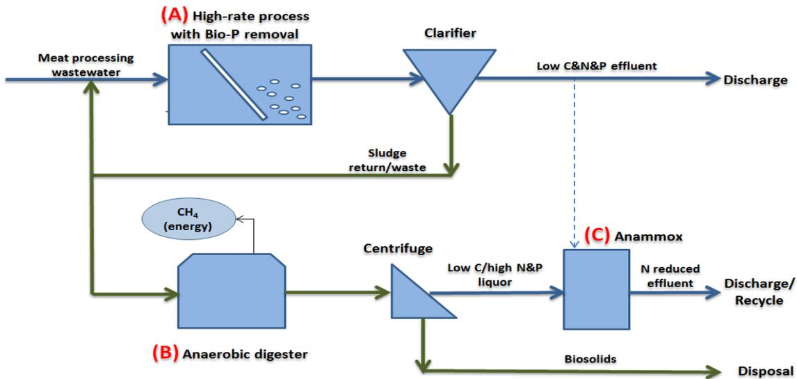
Figure 1: High-rate activated sludge process with integrated anaerobic digestion and anammox processes.
