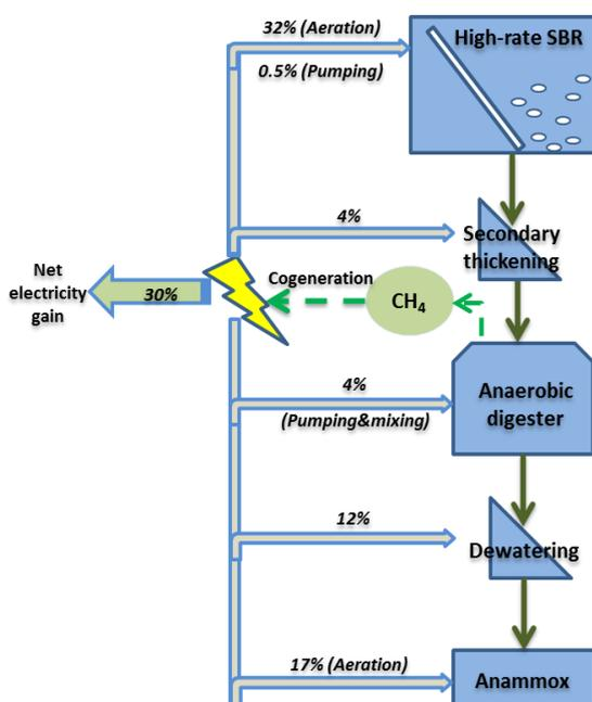
Figure 2: Flow scheme of potential electricity generation from the integrated high-rate wastewater treatment system.
