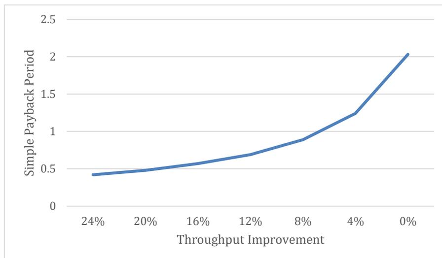
Figure 6: Impact of throughput improvement percentage on simple payback period.
