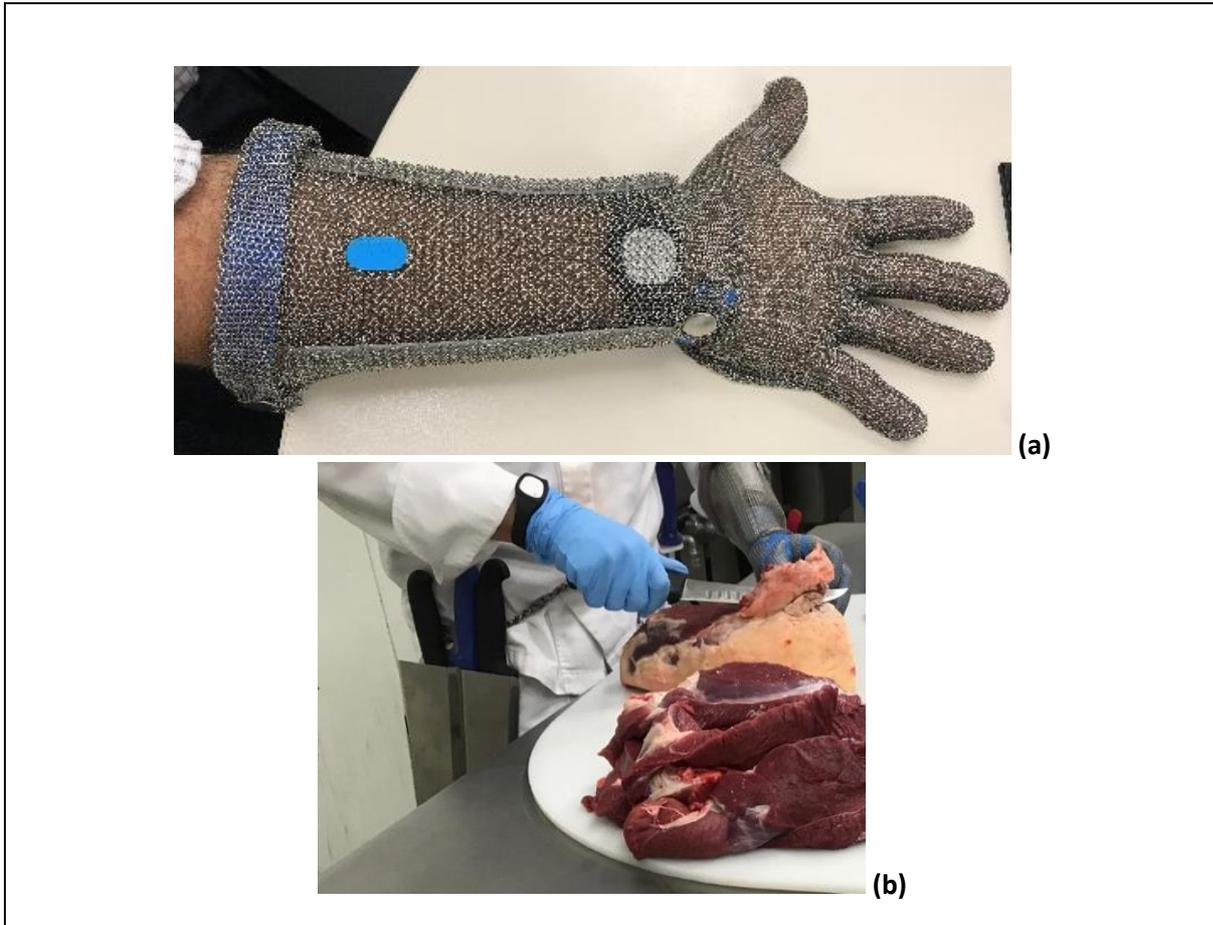
Figure 2: (a) IIoT Meta sensor (Watch Device) worn under protective mesh glove (b) Images from Pre-trial conducted at AMPC Industry Partner Plant
