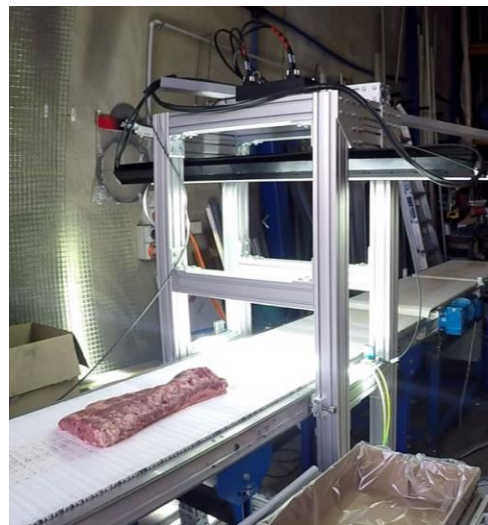
Figure 1: Primal cut recognition system equipment frame positioned over the product conveyor with a striploin
