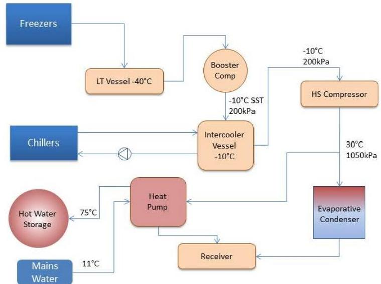
Figure 1 - AHP flow diagram
