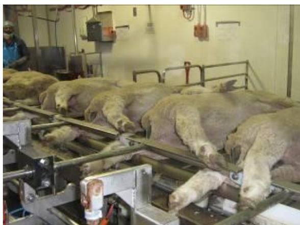
**Figure 1.** High frequency immobilisation used immediately post exsanguination and before the carcasses are placed on the chain. Source: E.S. Toohey
