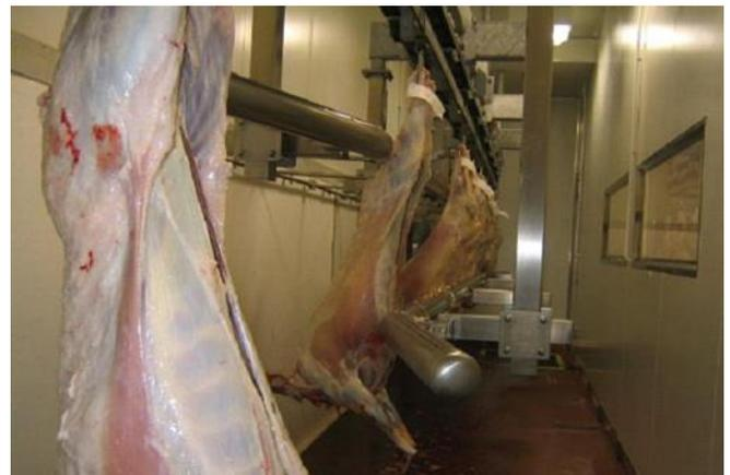
**Figure 4.** Post-dressing medium voltage electrical stimulation unit, bottom rail is active. Source: K. L. Pearce.
