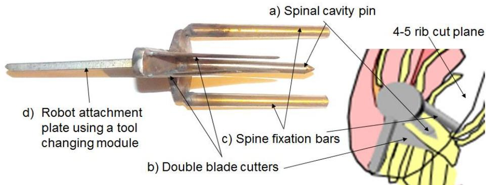
**Figure 4: Stage 1 fixation unit.**
