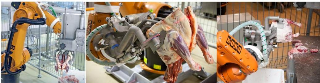
**Figure 8: Robot holds shoulder primal, driving it against fixed blades to perform de-boning (Scott Technology solution).**
