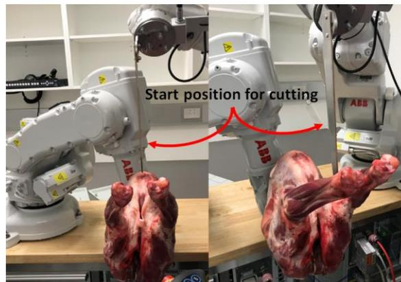
**Figure 18: Start of the ribcage boning process.**
