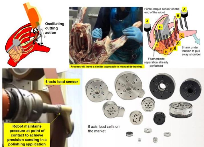
**Figure 13: Force control using a 6-axis load cell on the robot tool flange.**
