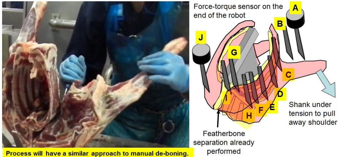
**Figure 14: Separation requirement to free the ribcage.**
