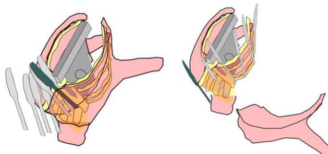
**Figure 10: Scheme for robotic de-boning.**
