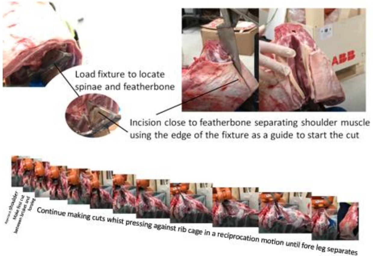
**Figure 15: Dry run with a robot.**
