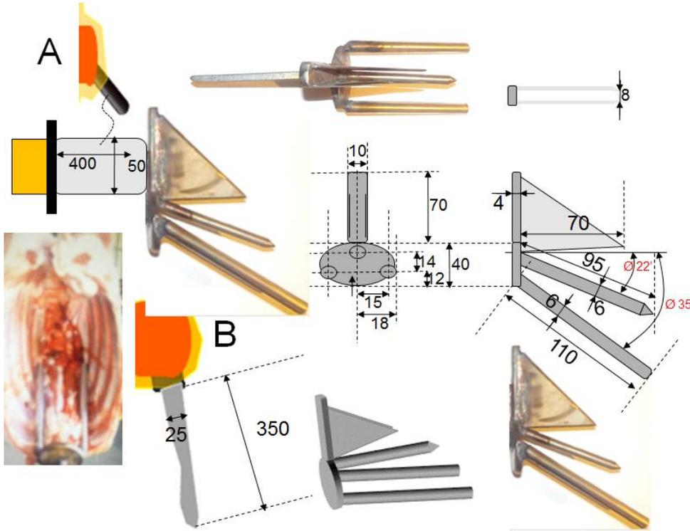
**Figure 12: Fixation details, robotic tools and primal piece locating.**
