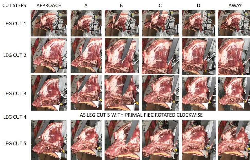
**Figure 20: Primal piece positioning by the handling robot and synchronised cutting.**
