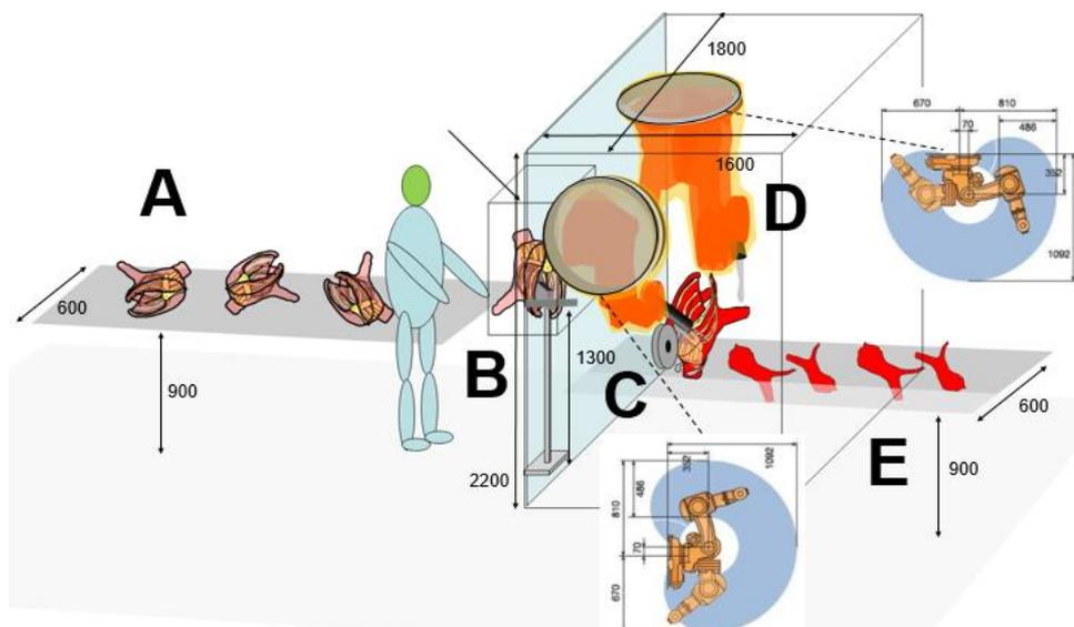
**Figure 3: Early concept for an automated twin Robot Cell for lamb shoulder de-boning.**
