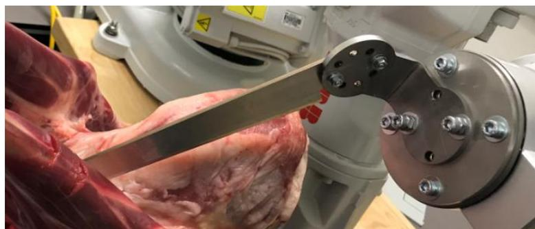
**Figure 16: The robot cutting knife.**
