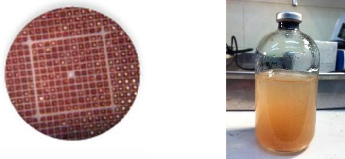
**Figure 4: The carrier with enriched anammox biomass collected from the parent anammox reactor (left), and the bottle setup for the specific anammox activity tests (right).**
