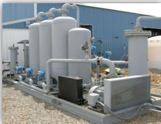
Figure 17: Skid mounted system to separate CO 2 from CH 4 in a biogas stream.
