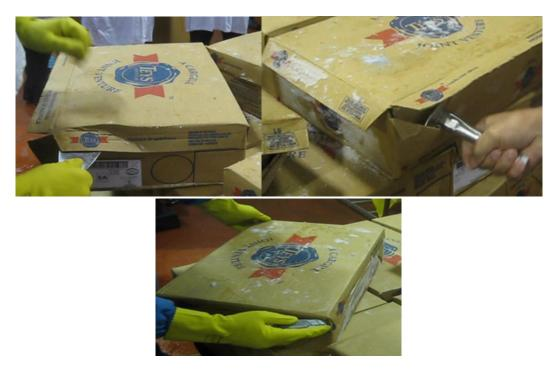
Fig. 8 Opening of linerless cartons after tempering using a commercially available spatula (a), purpose-built tool (b) or knife (c).
