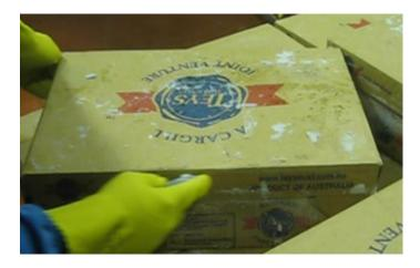
• Set Stanley knife to a depth of 8mm and run the knife edge along one long panel and the 2 short panels at about 5mm from the top.
