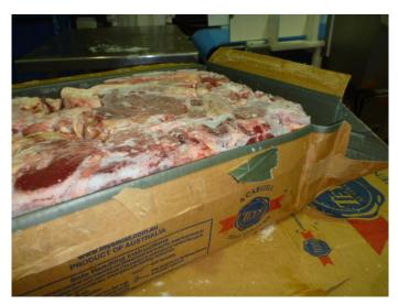
Fig. 5 Carton de-lidded showing delamination of the liner on the where it contacted glue on the carton lid.
