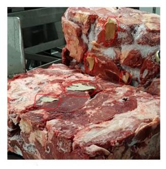
Fig. 9 Cardboard stuck to meat surfaces in de-boxed linerless carton meat.
