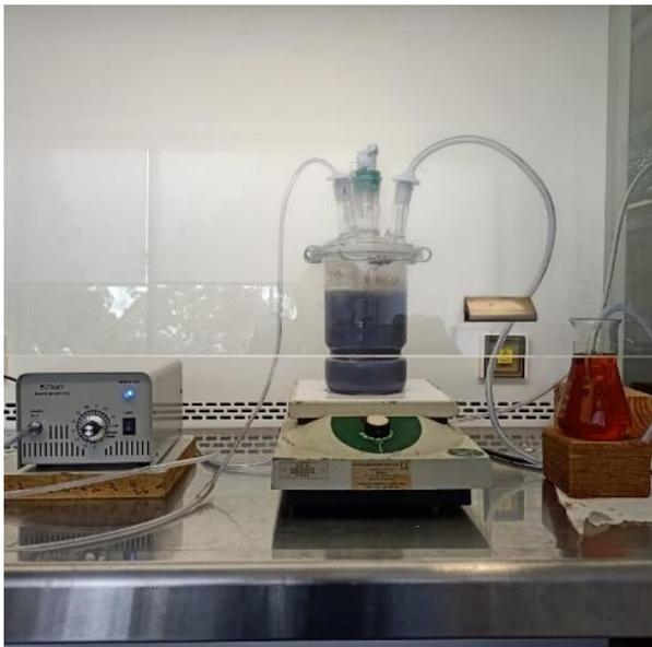
Figure 1. Lab setup showing ozone generator (left), reaction chamber (centre), and residual ozone trap (right).
