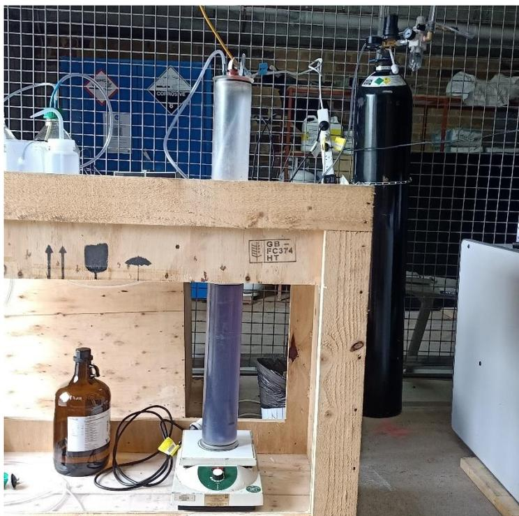
Figure 3. Modified lab setup showing elongated reaction chamber.
