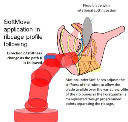
**Figure 8: SoftMove process for adaptation of separation path to ribcage profile.**
