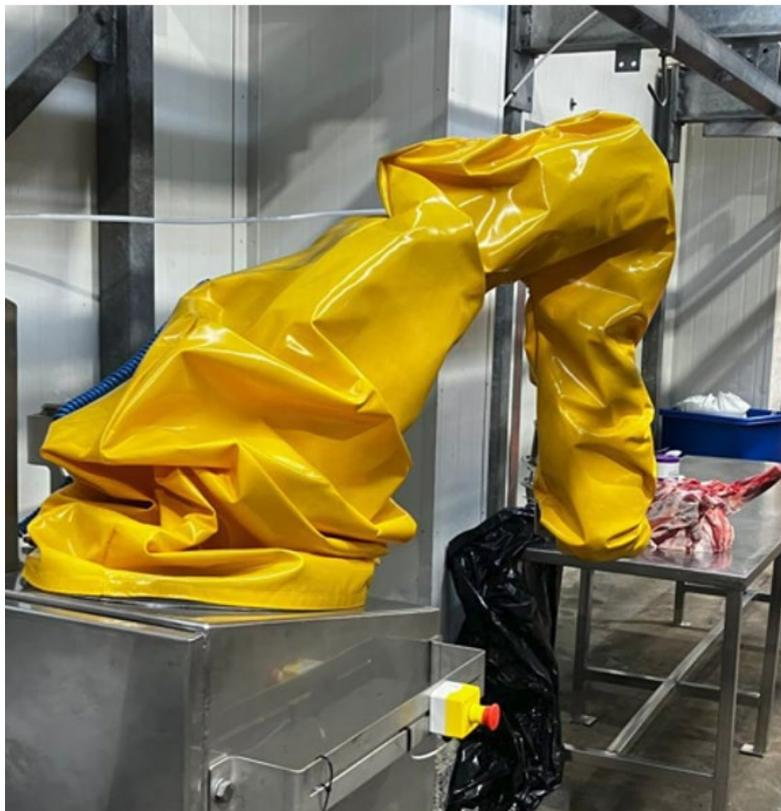
**World first integrated robot unit for forequarter ribcage separation, deboning of lamb shoulders.**
