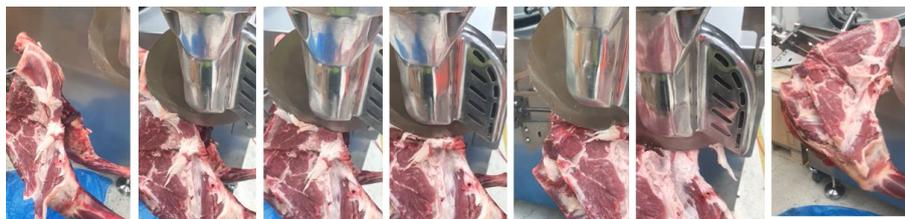
Motion (left to right) with ribcage in contact with blade, the robot, adjusting position perpendicular to the blade,
