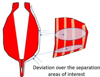
For a conforming FQ primal, the cut path over the separation areas away from the ribs, as shown, are to target a deviation not to exceeding 3mm for 85% of cuts and 5mm for all cuts.
