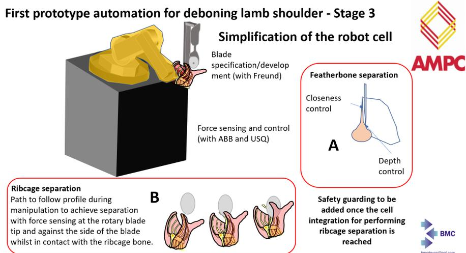
**Figure 6: Set-up to support developments for featherbone (A) and ribcage separation (B).**
