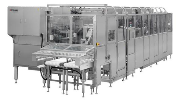
Mayekawa have developed an automatic deboning machine for pork hind legs capable of processing 500 legs per hour. The machine uses robots and various devices to cut and strip meat. It is not capable of deboning sow or beef legs.
