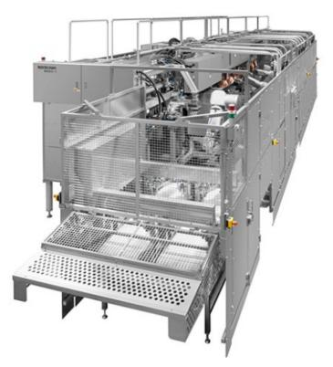
Mayekawa have developed an automatic deboning machine for pork fore legs capable of processing 600 legs per hour. The machine uses robots and various devices to cut and strip meat. It is not capable of deboning sow or beef legs.
