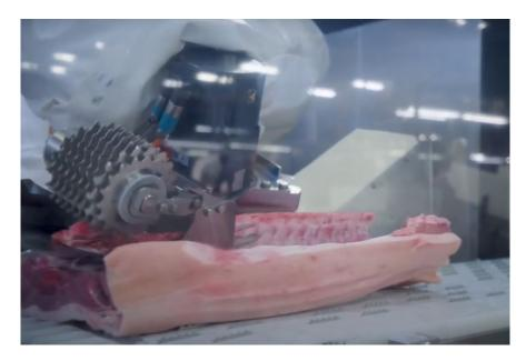
Frontmatec have developed a robot mounted circular cutting disc for pork chine bone cutting. Because product can move as it is cut, a planned cut path relative to product that is being cut could be difficult to achieve with good accuracy. Using a circular saw instead of a bandsaw enables the chine bone to be cut while the ribs are complete and the brisket is still attached to them.
