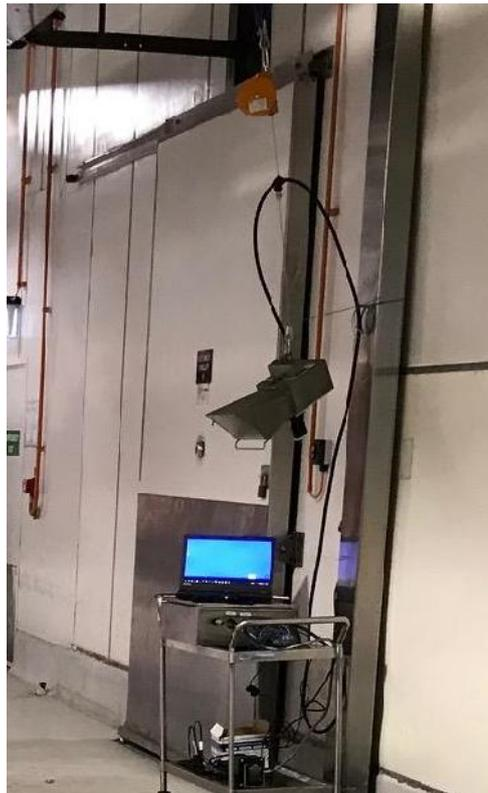
**Figure 2. The TenderSpec™ Beef Classification System ready for operation.**
