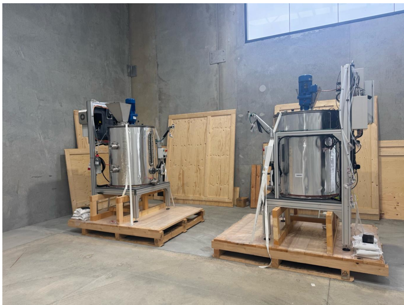
Figure 3. Reactors unpacked at Tessele Bio-Hub, ready for installation and wet commissioning.
