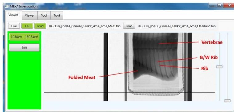
Figure 6 - MEXA transmission image of lamb rack with SCOTT software.
