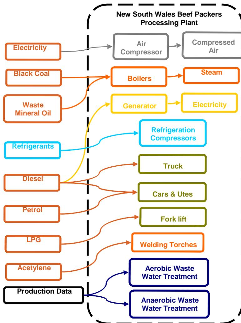
Figure 9 - NSW Processing Plant Revised Inputs Outputs Diagram
