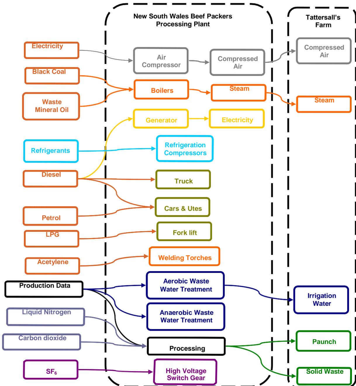
Figure 8 - NSW Processing Site Input Outputs Diagram
