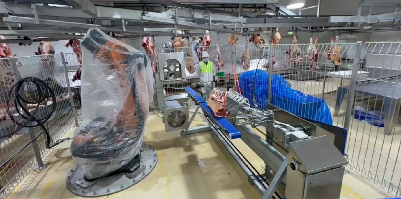
Figure 2: (Maunsell, 2024) Robotic Chining Cell
