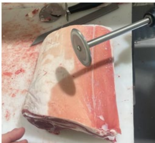
Figure 5 -Scribe Mark from Rotary Cutter attached to Drill. An extremely low force is required due to the rotating blade
