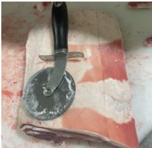
Figure 1 - Scribe Mark from Pizza Cutter. Line is visible but a medium force is required.
