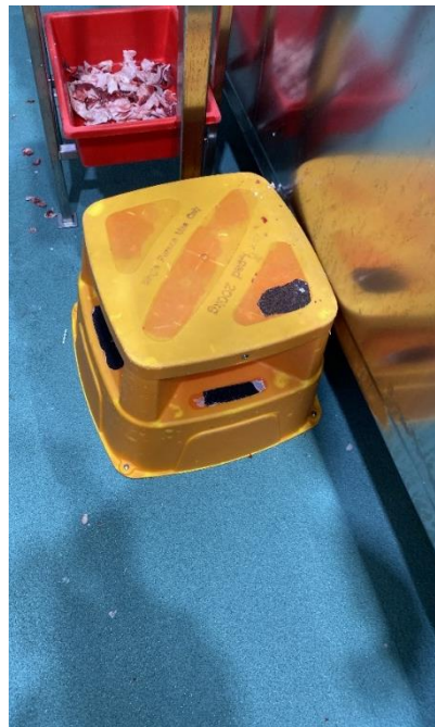
Fig 4. Step area too small to allow foot movement to minimize slip and fall risk.
