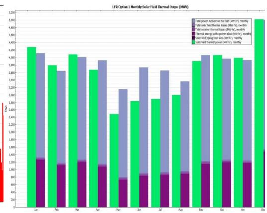
Figure 2 – Monthly Linear Fresnel solar field thermal output
