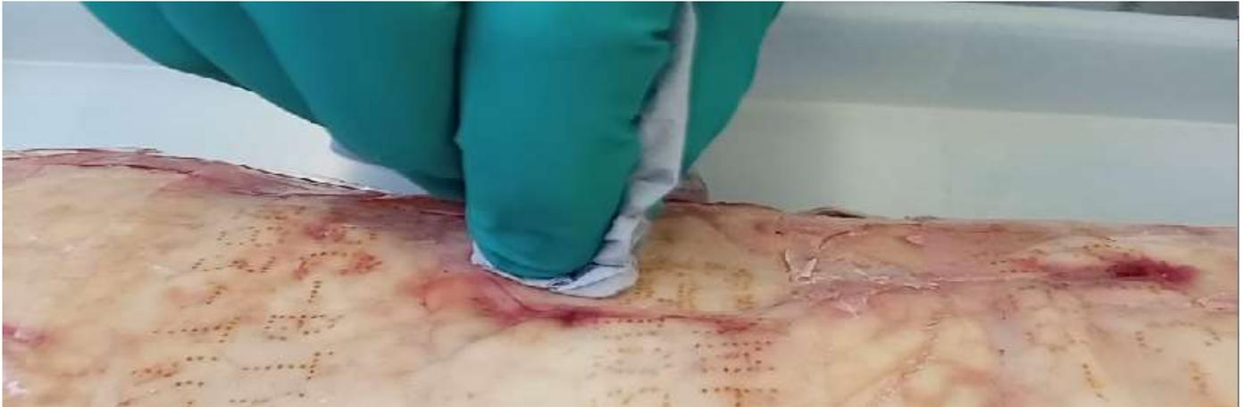
*Figure 36 Rub-test using paper towel to check adhesion of ink to fat*
