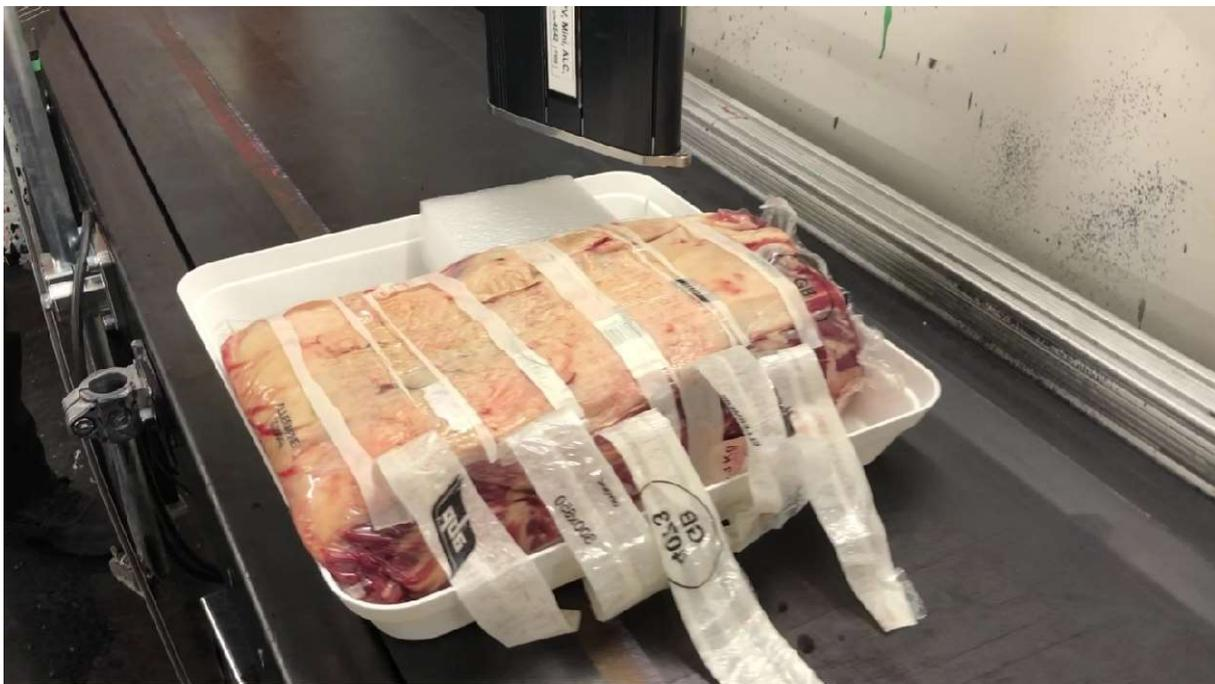
Figure 13 XACT printer setup, note the exposed areas of primal for printing and foam block
