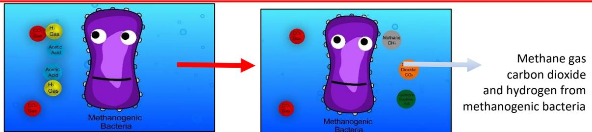
In the **third phase** methane producing bacteria convert the hydrogen and acetic acid produced by the acid forming bacteria into methane ( $CH_4$ ), hydrogen ( $H_2$ ) and carbon dioxide ( $CO_2$ ). The biogas exits the waste water and so the  $BOD_5$  and COD of the water are reduced.
