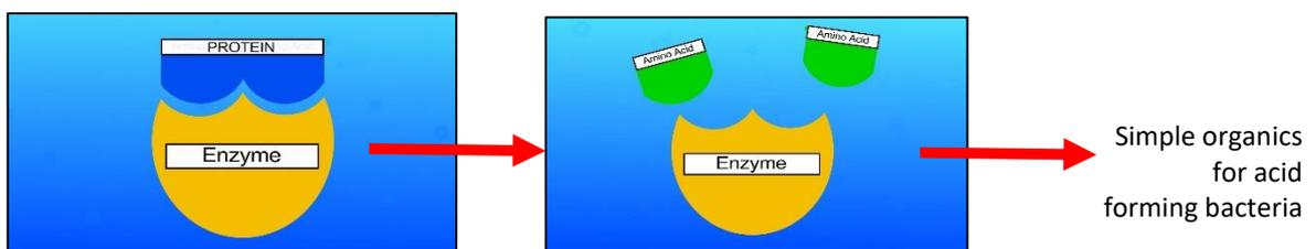
The **first phase** enzymes excreted from bacteria breakdown fats, proteins and carbohydrates in the wastewater into simpler water-soluble organics such as sugars, amino acids and fatty acids.
