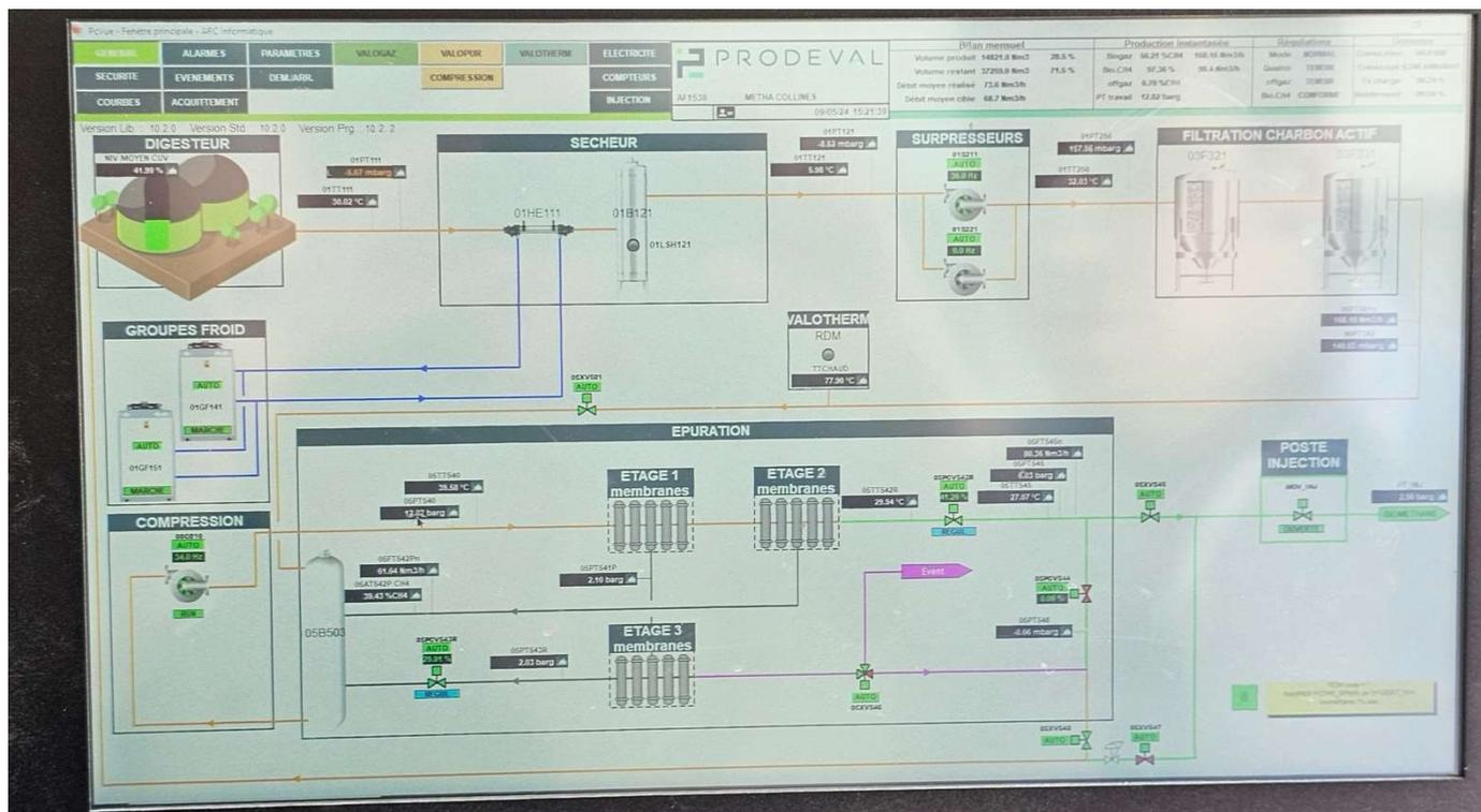
Figure 8. Screenshot with the process flow diagram at the Biodigesters and BioCO<sub>2</sub> recovery from agricultural residues and cow manure as feedstock in France.
