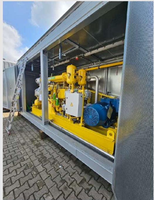
Figure 1. Images from the ETW manufacturing facilities, focused on biogas upgrade and liquid CO2 recovery.
