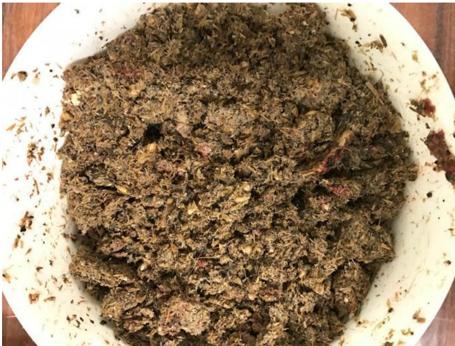
Figure 40 RMP4 – Example of Screened and Dewatered Red Solids from primary treatment at RMP plant 1
