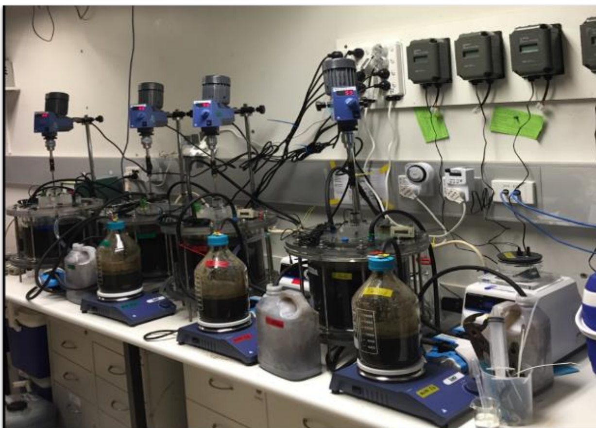
Figure 8: Four continuous bench-scale digesters constructed and operated to test organic loading limits for a complex base substrate co-digested with model co-substrates
