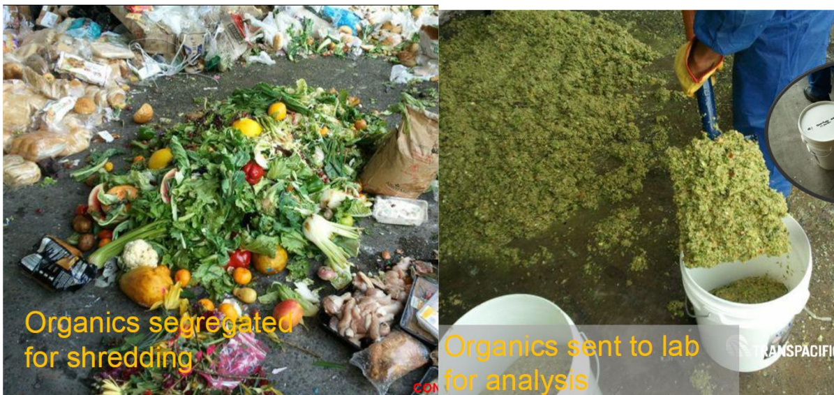
Figure 36: SFW1 – Example of Food waste used in BMP testing, separated prior to maceration (extracted from Cleanaway presentation to QUU).
