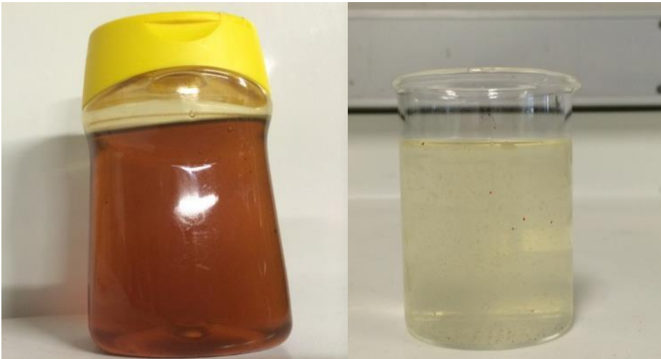
Figure 45: FIO2- Sample of wastewater from a honey processing plant, compared to honey. Waste was supplied by QUU.
