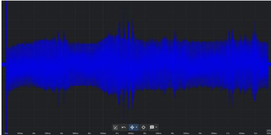
Figure 20 - Current draw when performing rib cuts
