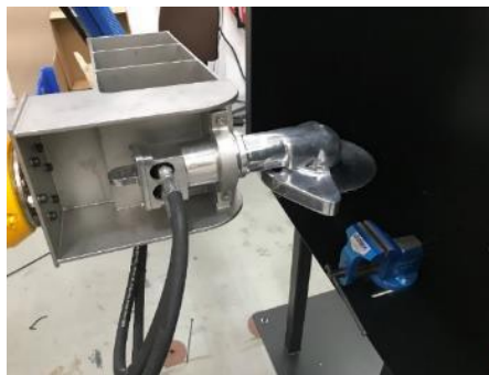
Figure 10: Saw Mounted to End Effector
