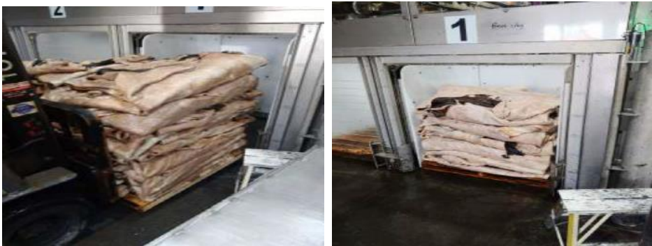
Figure 3 - Example of Palletised Hides exiting the palletiser
