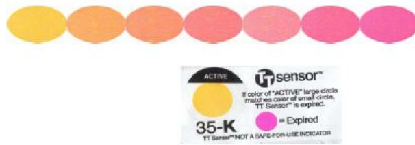
Figure 9. The TT Sensor™ diffusion-reaction Time-Temperature Indicator (Avery Dennison Corp.: USA).
