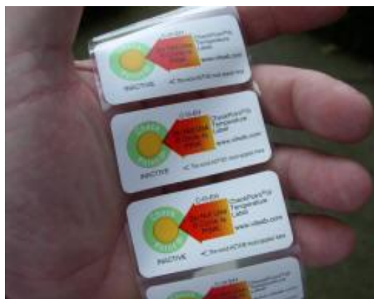
Figure 10. The CheckPoint® Time-Temperature Indicator which suggests ‘do not use if the circle is pink’ (Vitsab International: Sweden)
