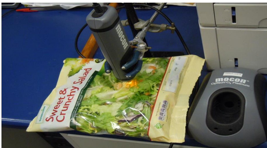
Figure 6. The Optitech™ OxySense® developed by LUXEL Biosences Ltd, University College Cork and MOCON, USA
