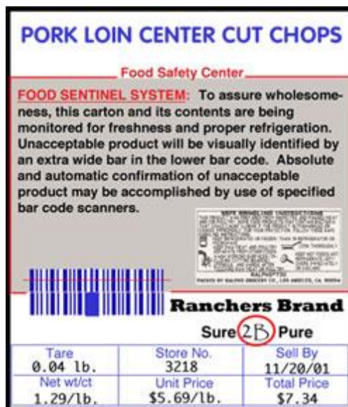
Figure 7. The SIRA Technologies Inc. Food Sentinel System™ whereby contaminating bacteria render the barcode unreadable.
