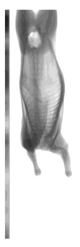
Figure 2-4- Calibration Block Reference next to Lamb Carcass
