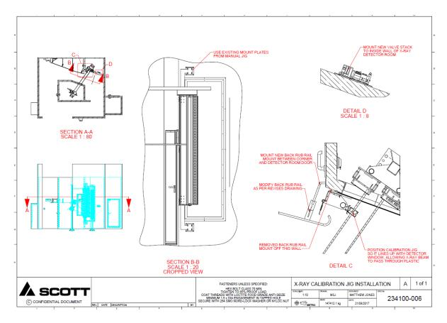
Figure 2-6- X Ray Calibration Jig Installation after Modifications
