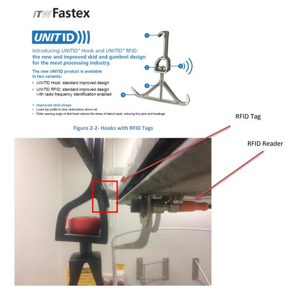
Figure 2-3- RFID Tag and Sensor
