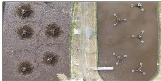
In **Sequence Batch BNR processes**, nitrification and denitrification occur in the same reactor space, but at different times in the cycle. For example, the aeration system turns on for the nitrification part of the cycle, then switches off during the denitrification period. This saves the need for pumping large volumes of liquid around or for separate structures such as clarifiers.
