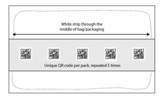
Concept Design for fixed length pre-printed primal shrink bag for traceability with repeated codes and white strip. © Trust Codes Limited 2022.
