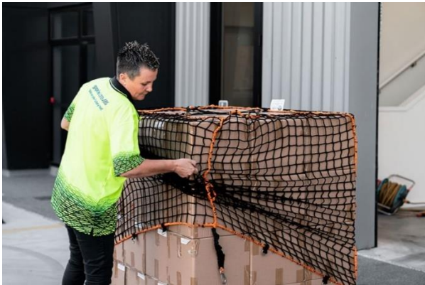
Figure 5.6.1 - Pallet netting being installed by an operator (Source: https://palletnets.com/ )
