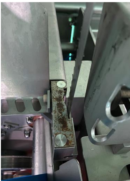
Image 7. Bandsaw blade guides need replacing regularly
