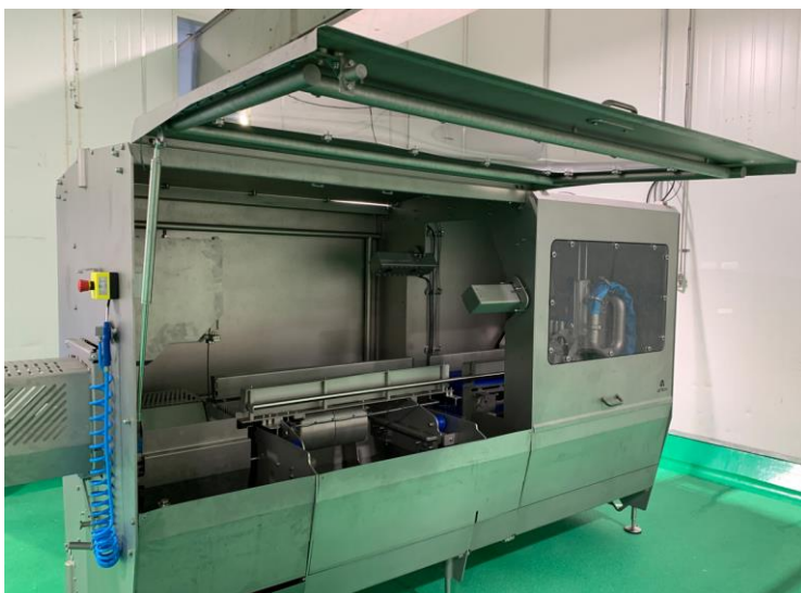
Image 5. Side panels lift on hydraulics for easy access
