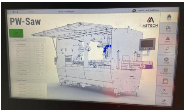
Image 4. User interface touch screen programme variables
