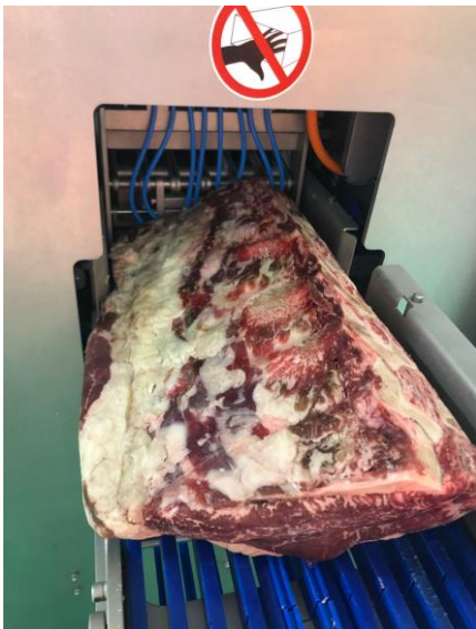
Image 13. The input belt width is 260mm wide.
