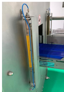
Image 16. Infeed belt sensor gate
