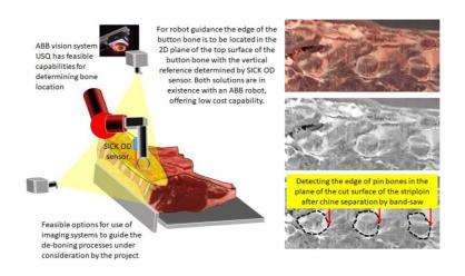
Figure 6: Vision sensing enhanced by OD and touch sensing keeping solution costs low, using proven and feasible capabilities.
