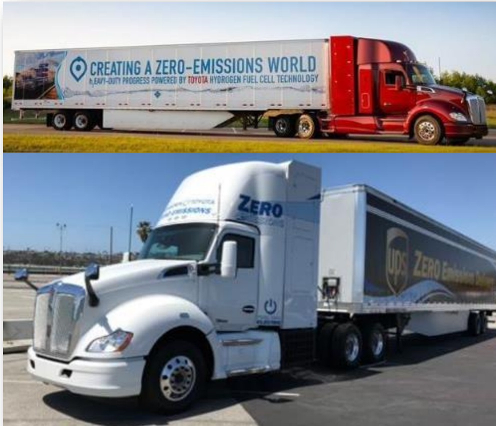
Figure 10: Kenworth T680 outfitted with a hydrogen fuel cell electric powertrain from Toyota. The truck uses two of the standard car fuel cells.
