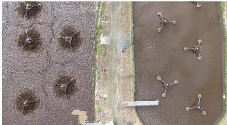
Image 19: Sequencing Batch Reactors
