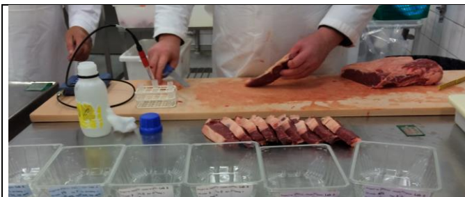
Picture 5. pH measurement and cutting of steaks
