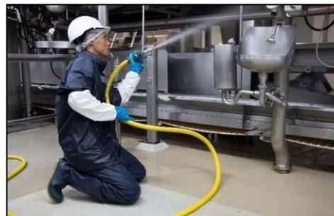
The majority of wastewater is generated from cleaning and sterilising equipment.
