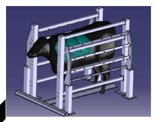
Figure 2: Intelligent Animal Cleaning Device – Final Design Concept (RMIT 2018)
