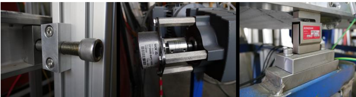
Figure 9: Frame bolts to attach to conveyor (left), encoder setup with motor coupling and mount (middle), load cell holding up conveyor and attached to base frame (right)
