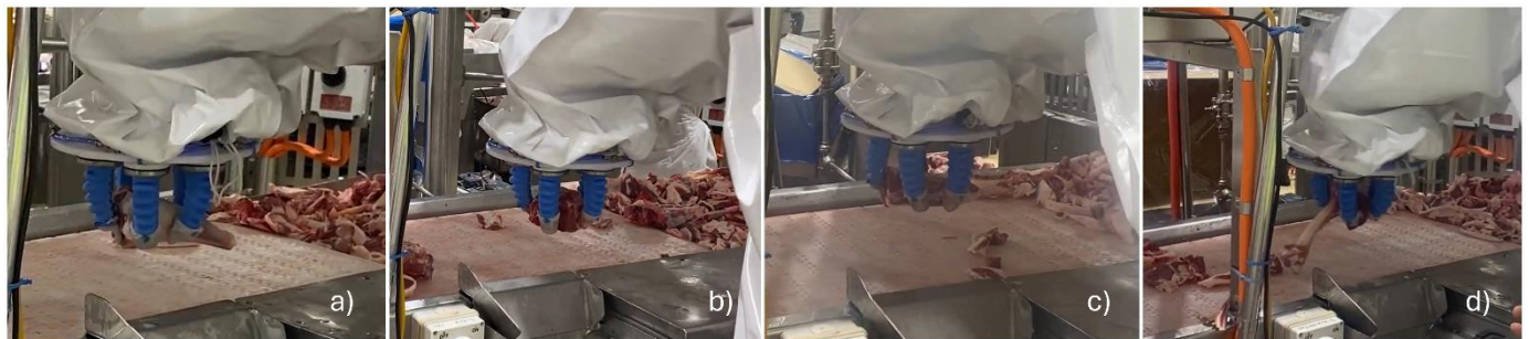
Figure 6: Images of successfully picked lamb products by the shadow robot. a) shank, b) neck, c) breast piece, and d) femur bone.
