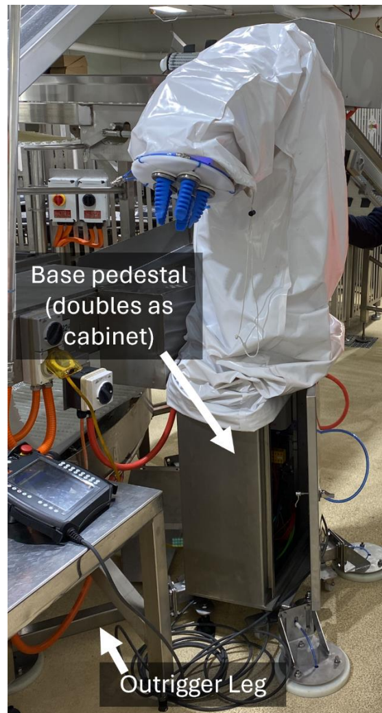
Figure 3: Photo of the shadow robot and associated base where the pedestal cabinet and outrigger legs are visible.
