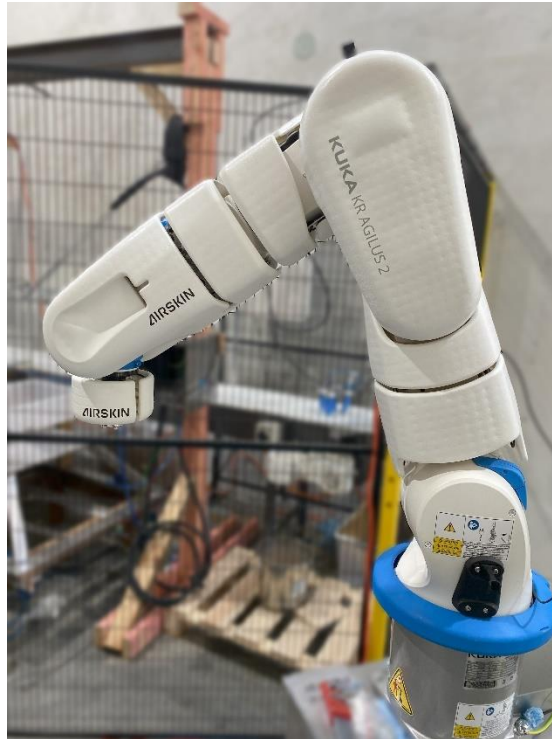
Figure 4: Shadow robot with AIRSKIN® safety system installed.
