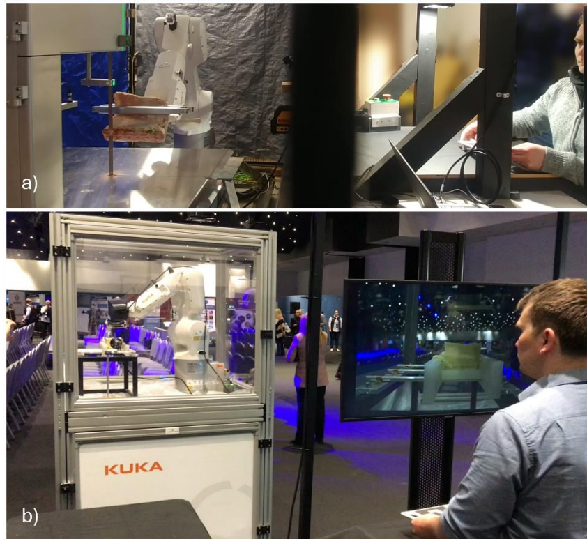
Figure 1: Photos of the shadow robot system being demonstrated during Stage 2 to perform a) a chine cut and b) trimming.
