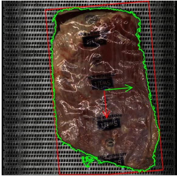
Figure 16: Processed Recitified image with region of the found primal cut (green outline), bounding box (red rectangle), pick position and rotation identified by coordinate arrows.
