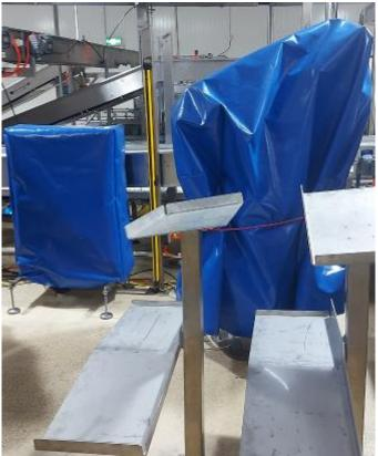
Figure 10: Washdown covers for camera and lights (left), control cabinet and robot (right)
