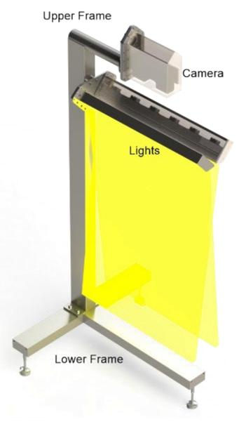
Figure 8: Rendering of camera and lights frame design. Camera and light covers are transparent to show details of the camera and lights respectively.
