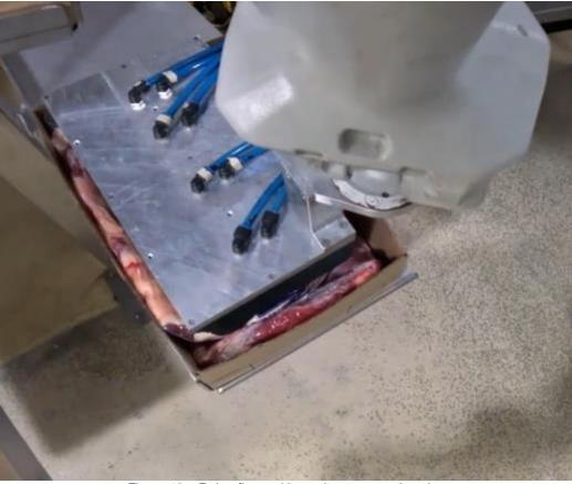
Figure 18a: Robot flat packing to lower carton location.
