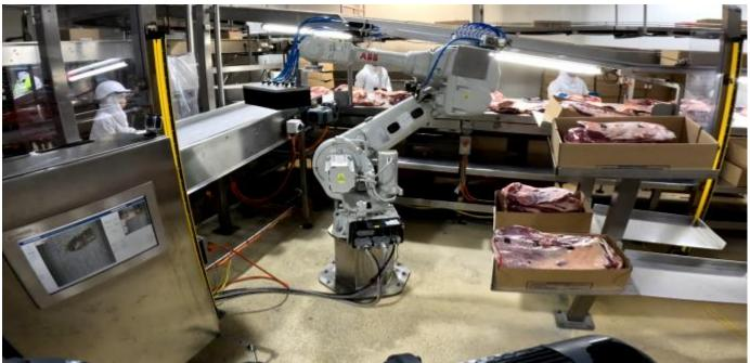
Figure 20: Robotic Picking and Packing system operating during in-plant trial.
