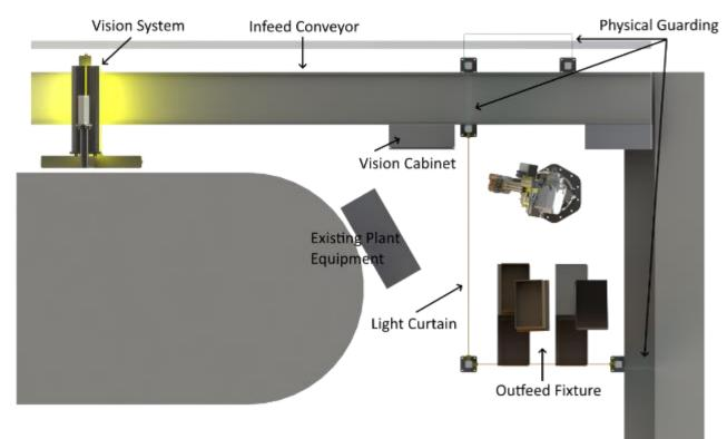
Figure 11: Cell Layout rendering, overhead view.
