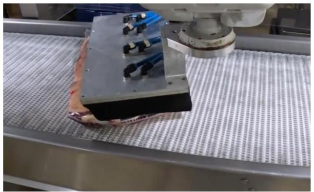
Figure 17a: Robot picking showing rotation based on primal cut angle relative to conveyor.
