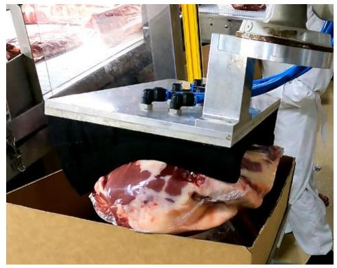
Figure 16b: Robot flat packing to upper carton location.
