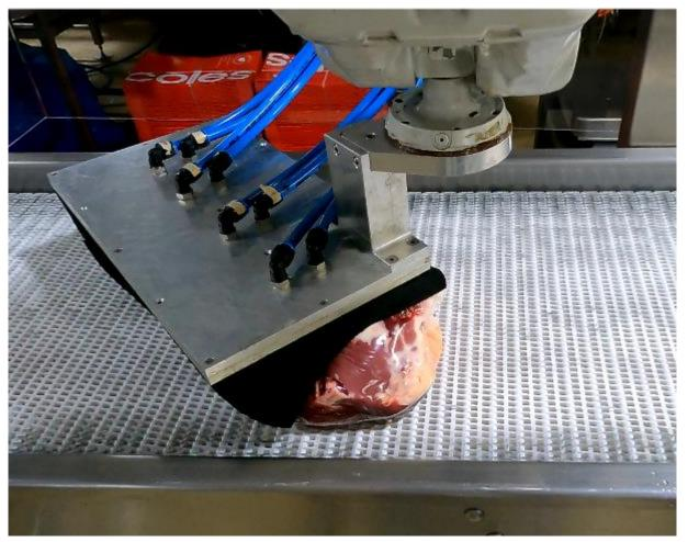
Figure 15b: Robot picking showing rotation based on primal cut angle relative to conveyor.
