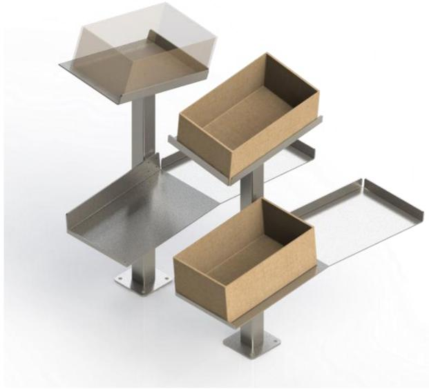
Figure 9: Packing carton outfeed fixture.
