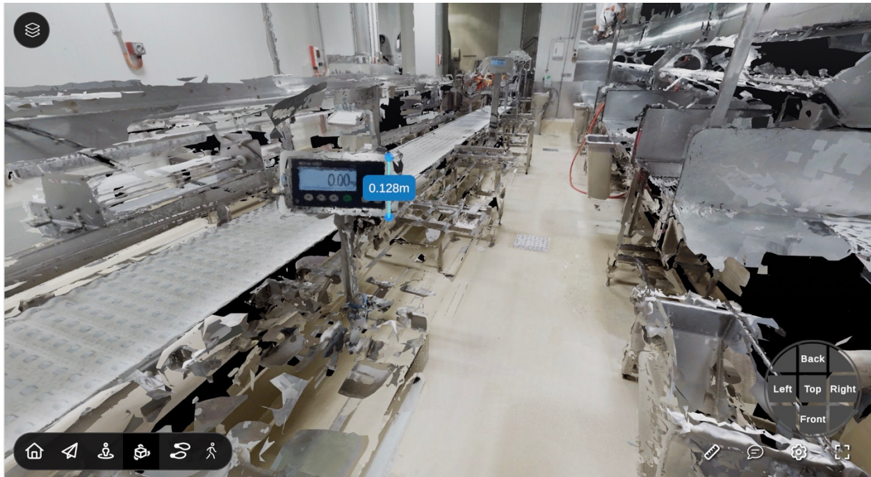
Image 2.3 – The Offal Room as a meshed 3D output, struggling with the reflections. But still able to be accurately measured.
