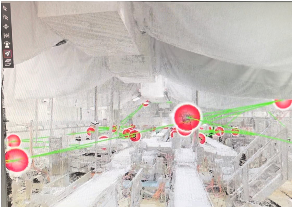
Image 2.1 – Original outputs from the LIDAR: a colourized pointcloud. .
